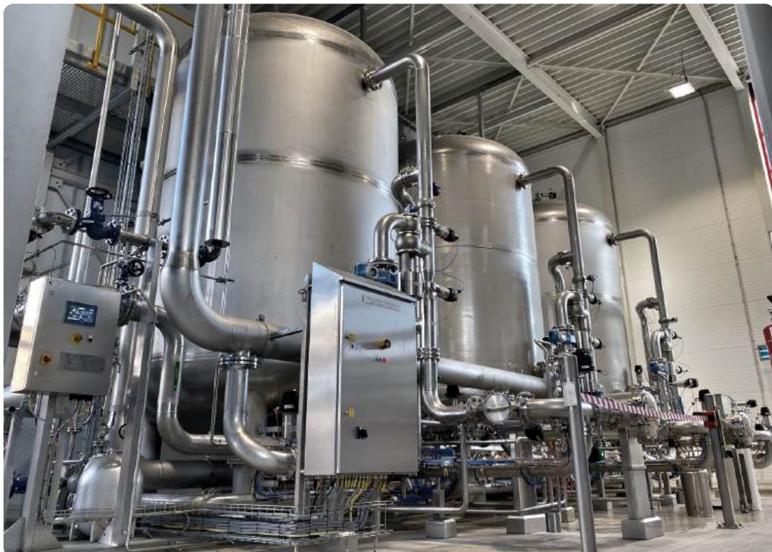
Complete activated carbon treatment and downstream polishing filtration system.
